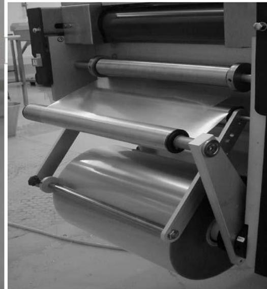
**Fig A2.1 Thermoforming machine<sup>1</sup> (Multivac R230 thermoform fill seal machine)**      **Fig A2.2 Plastic entry detail**
