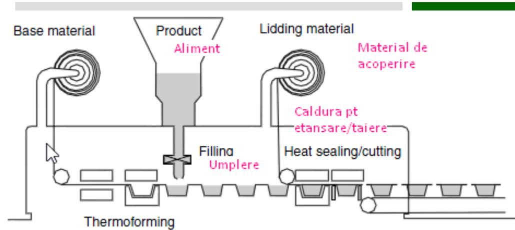
The lower foil is fed from a bobbin and heated prior to molding or molding, then the foil is molded by various processes. The cavity thus formed is filled with the food in an open atmosphere or vacuum, after which the upper foil is used for closing, which due to heat and pressure is welded to the airtight lower foil. Cutting devices are used to divide finished products. It follows product labeling and evacuation.
