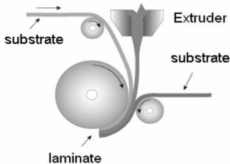
Fig.3 Coating and lamination by extrusion, according to
