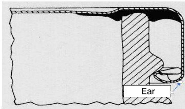
**Pressure and twist opening cap Fig. 7 (PT-Press-on Twist-on Cap)** consists of a non-ear steel case. The seal is made of molded plastic that covers a sealing area extending from the top outer edge of the lid to the curvature of the cap, forming the primary top seal and a secondary seal on the side.
