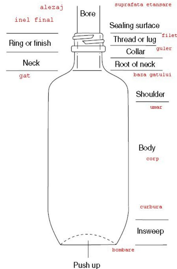
Fig 5. Components of a glass bottle. According to RICHARD COLES, DEREK MCDOWELL, MARK J. KIRWAN FOOD PACKAGING TECHNOLOGY, Blackwell Publishing Ltd, 2003
