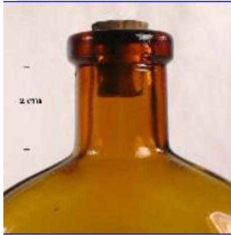
**The cork stopper** is the most common and most traditional glass bottle sealing device. It comes from the bark of the cork tree that grows in SE Europe and Africa. Cork elasticity the ability to keep its normal size after compression - was the basic property of the stopper, allowing it to be squeezed into a bottle's bore and create a gasket. In addition, its chemical inertia has made it ideal for sealing almost any type of bottled product - liquid or solid - without giving it a flavor.
