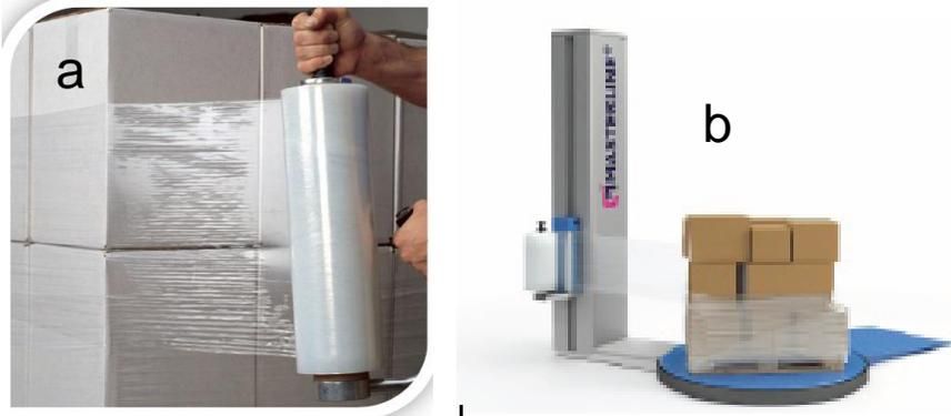
Fig 2 Manual stretch film (a) (<http://luckapack.ro>) and automatic(b) [www.antal.ro](http://www.antal.ro)
