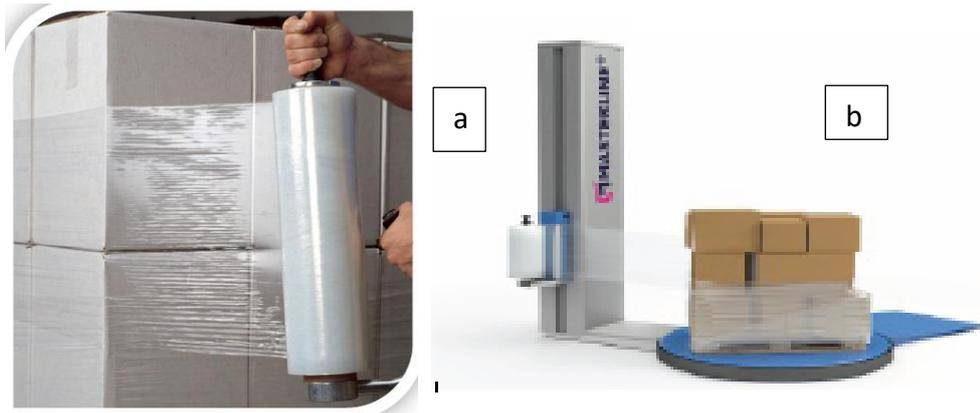
Fig 2 Manual (a) (<http://luckapack.ro>) and automatic (b) [www.antal.ro](http://www.antal.ro) stretch film
