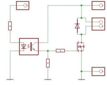
**IMAGE 10: THIRD CONTROL CIRCUIT PROTOTYPE WITH MOSFET TRANSISTOR.**
