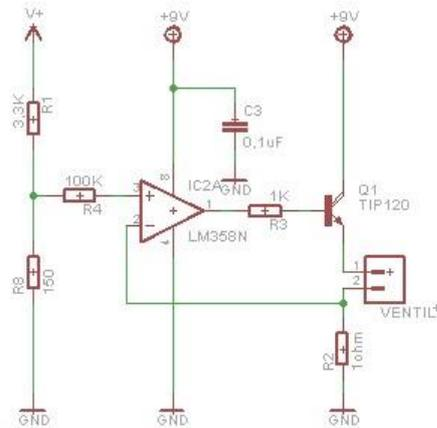
**IMAGE 6: VALVE CONTROL CIRCUIT.**
